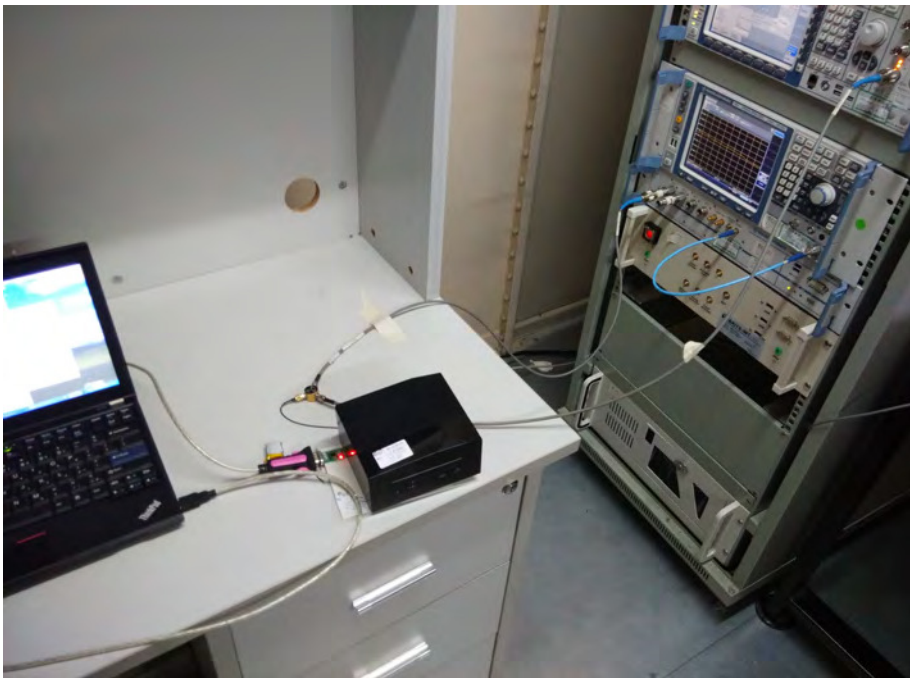
Conducted Test Bluetooth 3.0
