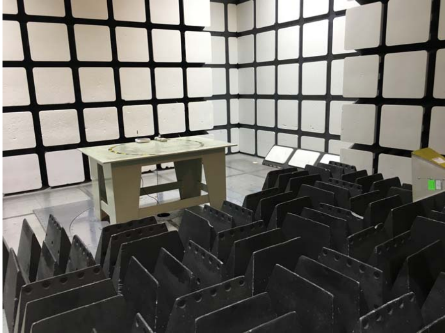
Radiated Emissions – Front View (Above 1 GHz)
