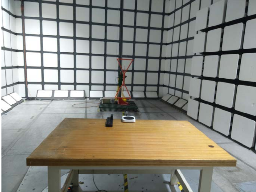
Radiated Emissions – Front View (Below 1 GHz)
