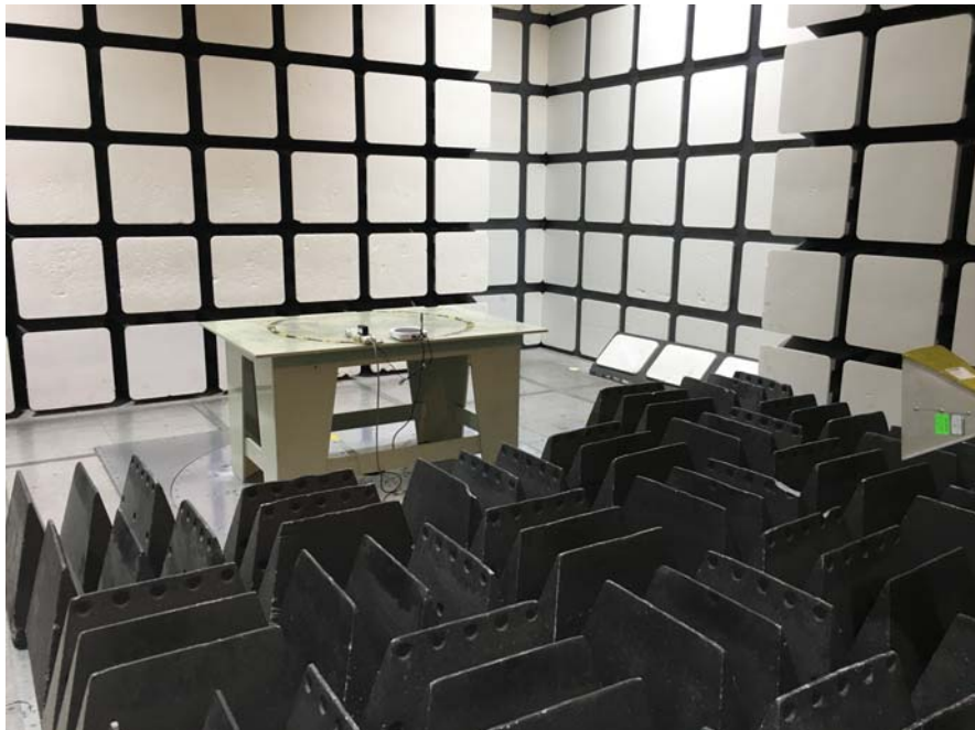
Radiated Emissions – Rear View (Above 1 GHz)
