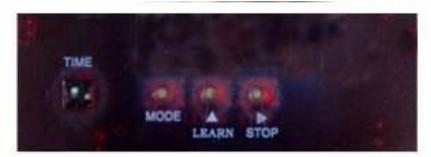
If you selected Clock function, after you press "Stop", you can set the time, press "Learn" to adjust the number, when the number is right, press "Stop" to switch to next number. The rest can be done in the same way. Then the screen will show calling number and present time alternately.
