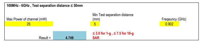
In addition , the maximum transmission duration reading single tag is 10msec , and 350msec for reading multiple tags,. Per KDB 447498 Section 5.3 , the max duration of overlapping transmission of EUT with cell phone will be less than 30 sec. therefore , simultaneously transmission RF exposure evaluation is no needed.
