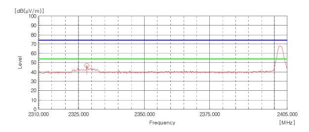
AV Detector: RBW: 1 MHz, VBW: 10 Hz (2 310 MHz - 2 390 MHz), Worst case (Low, Horizontal)
