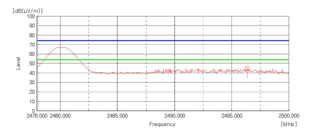
AV Detector: RBW: 1 MHz, VBW: 10 Hz (2 483.5 MHz - 2 500 MHz), Worst case (High, Horizontal)
