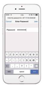
Now the iPhone is connected to the Dongle. Drag out the below menu from the bottom of the screen, we can see the Airplay icon, see below picture:
