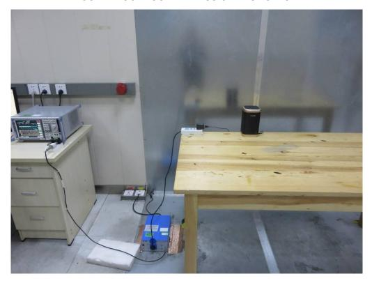
FCC RADIATED EMISSION TEST SETUP
