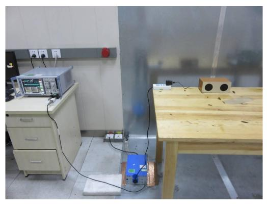
FCC RADIATED EMISSION TEST SETUP
