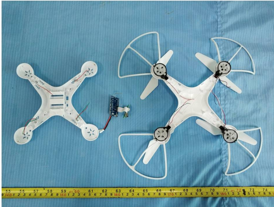
EUT – Cover off View 3
