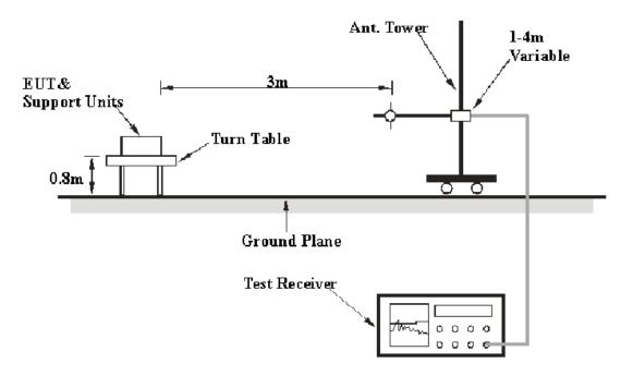
The radiated emission tests were performed in the 3 meters, using the setup accordance with the ANSI C63.10-2013. The specification used was the FCC Part 15.205 and 15.209 and 15.227 limits.
