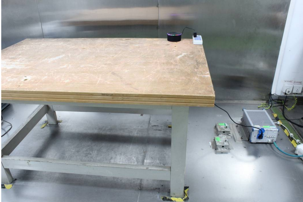
Conducted Emissions - Front View
