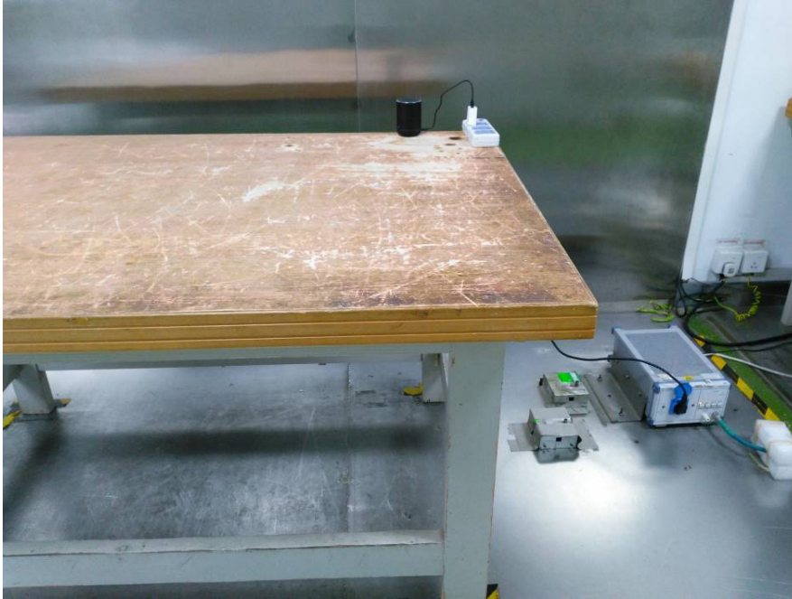
Conducted Emissions - Front View
