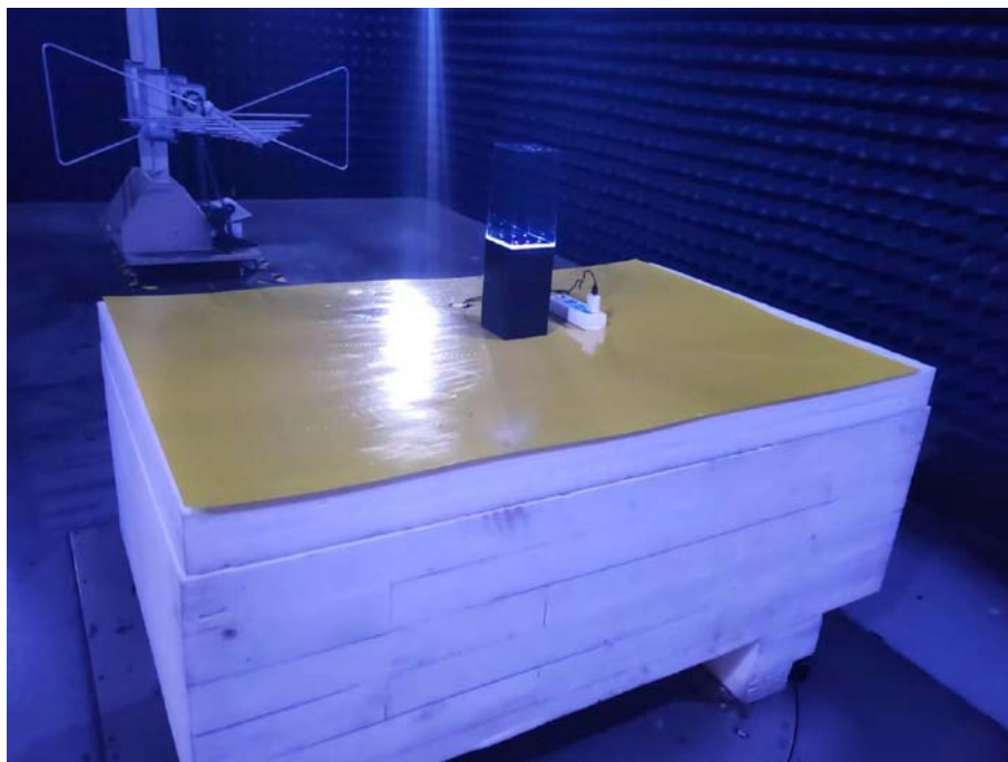
Photo of Radiated Emission Measurement Below 1GHz
