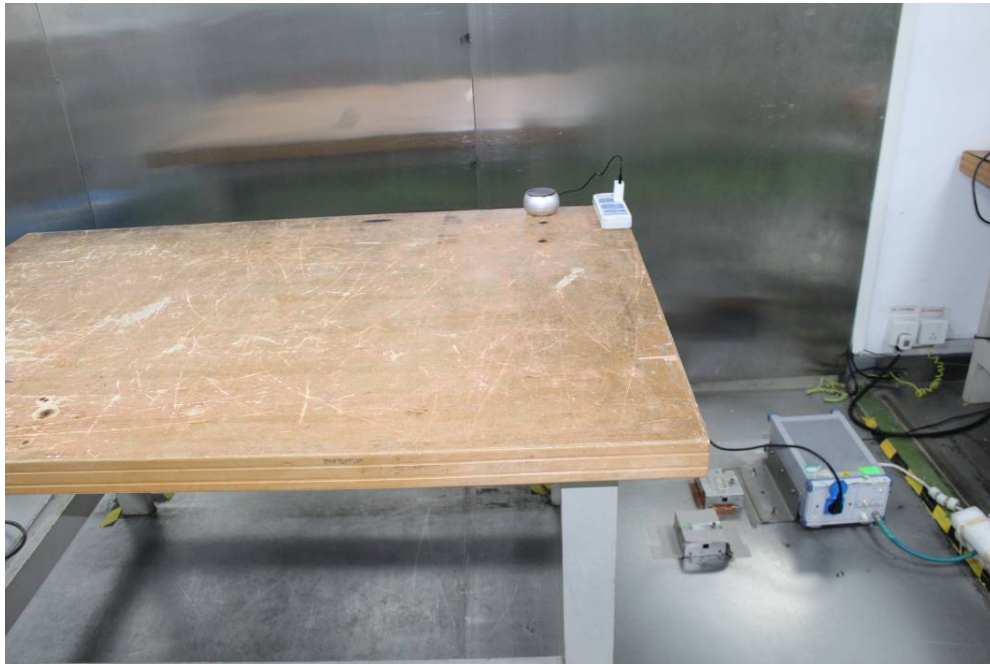
Conducted Emissions - Front View
