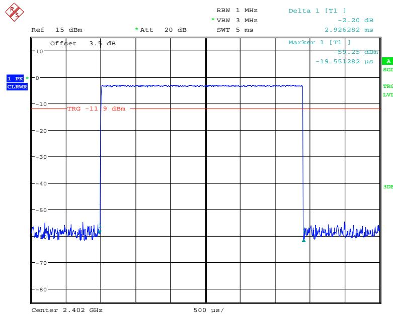
**Pulse time, Middle Channel, DH5**
