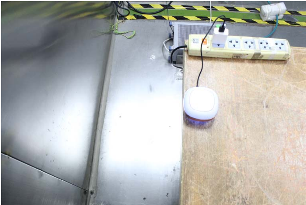
Conducted Emissions - Side View
