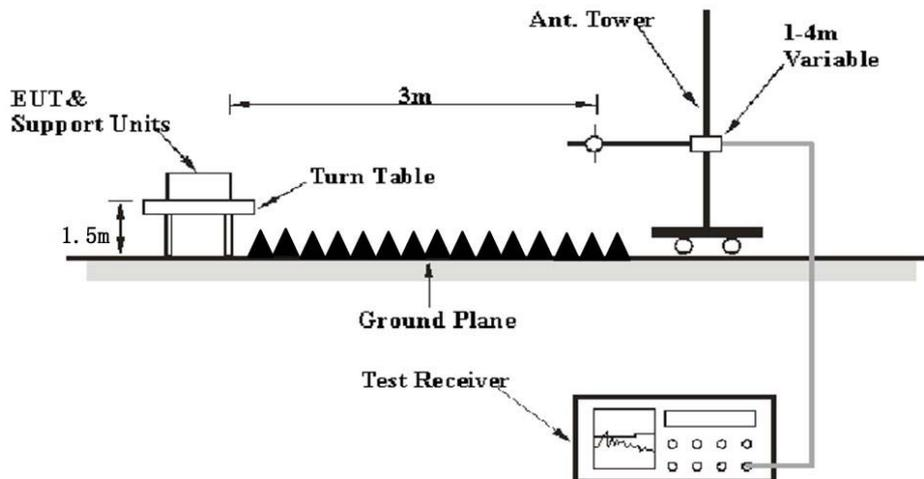
The radiated emission tests were performed in the 3 meters, using the setup accordance with the ANSI C63.10-2013. The specification used was the FCC 15.209 and FCC 15.247 limits.
