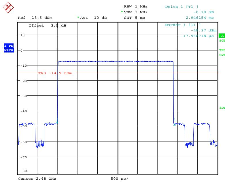
**EDR ( $\pi/4$ -DQPSK):****Pulse time, Low Channel, 2DH1**
