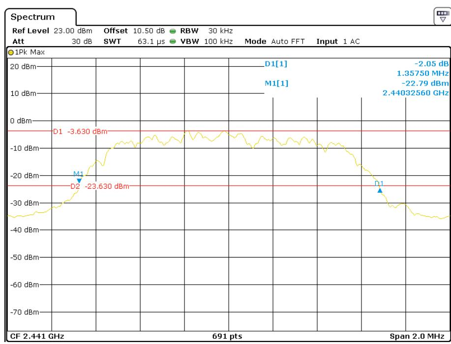
**EDR ( $\pi/4$ -DQPSK): High Channel**
