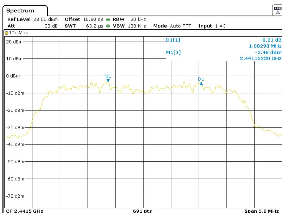
**EDR (8DPSK): High Channel**
