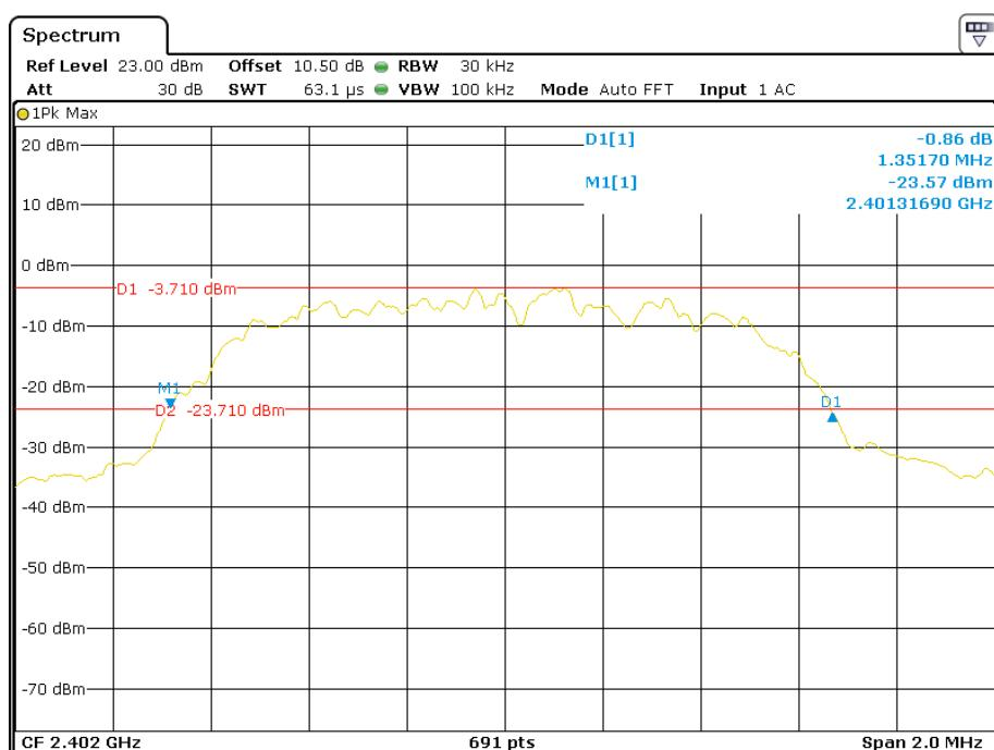
**EDR (8DPSK): Middle Channel**
