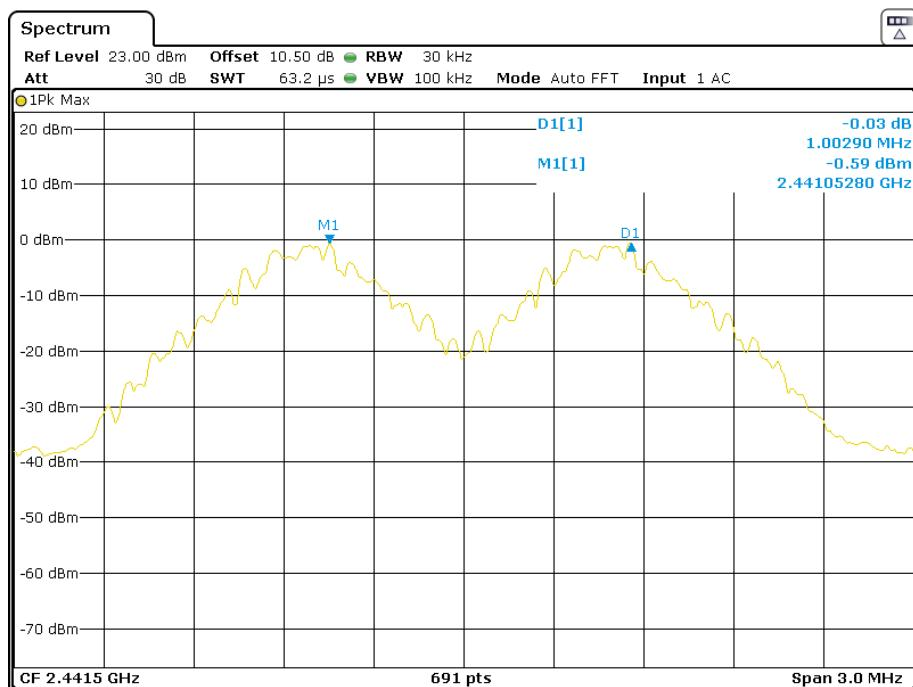
**BDR (GFSK): High Channel**
