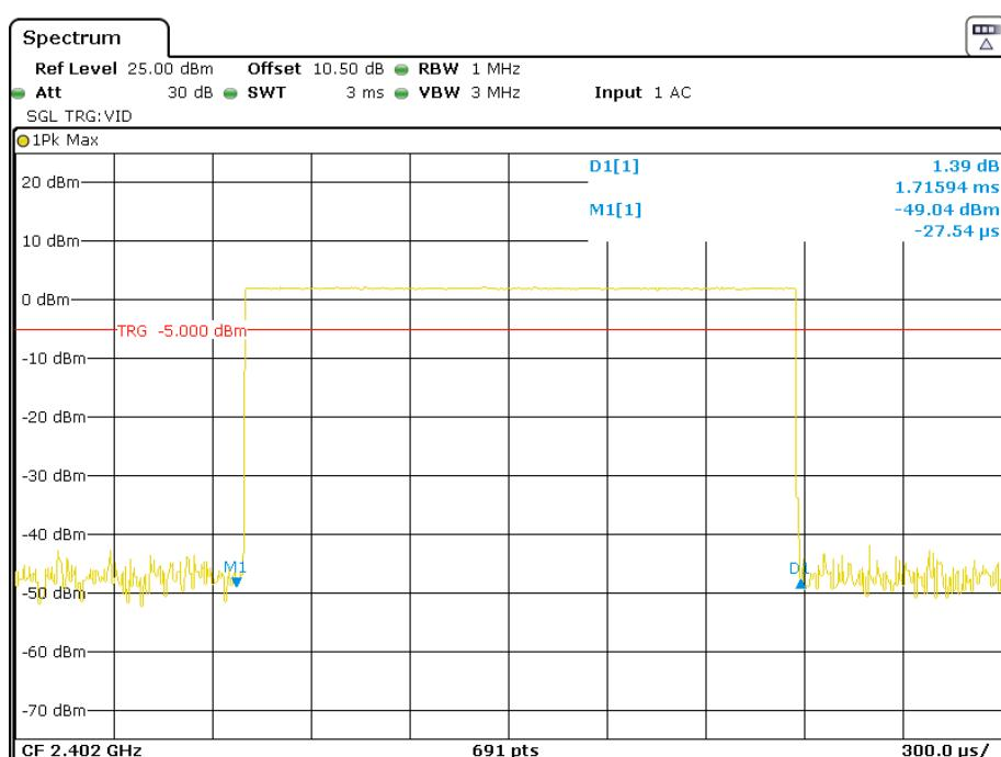
**Pulse time, Middle Channel, DH3**
