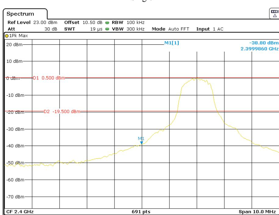
**EDR ( $\pi/4$ -DQPSK): Band Edge-Right Side****Hopping**
