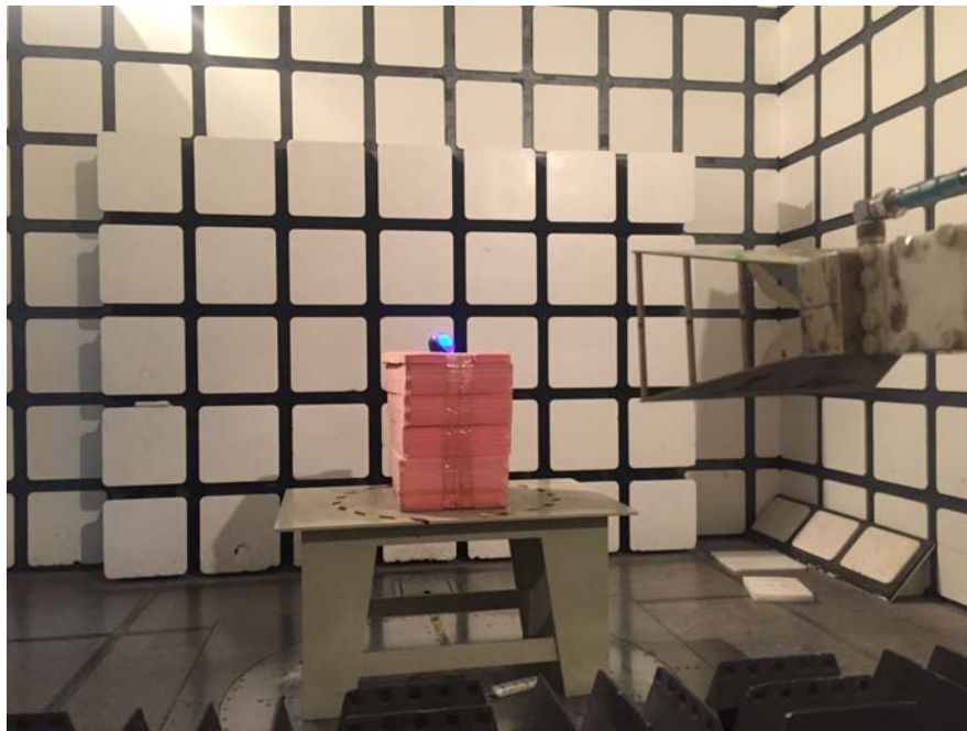
Radiated Emissions View (Above 1 GHz)
