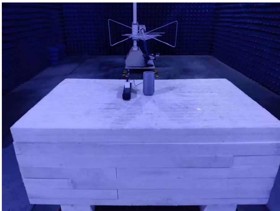
Photo of Radiated Emission Measurement Above 1GHz
