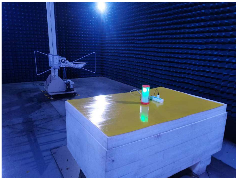
Photo of Radiated Emission Measurement Below 1GHz
