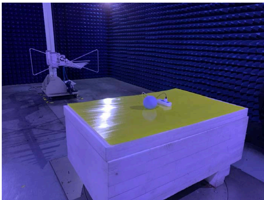
Photo of Radiated Emission Measurement Above 1GHz
