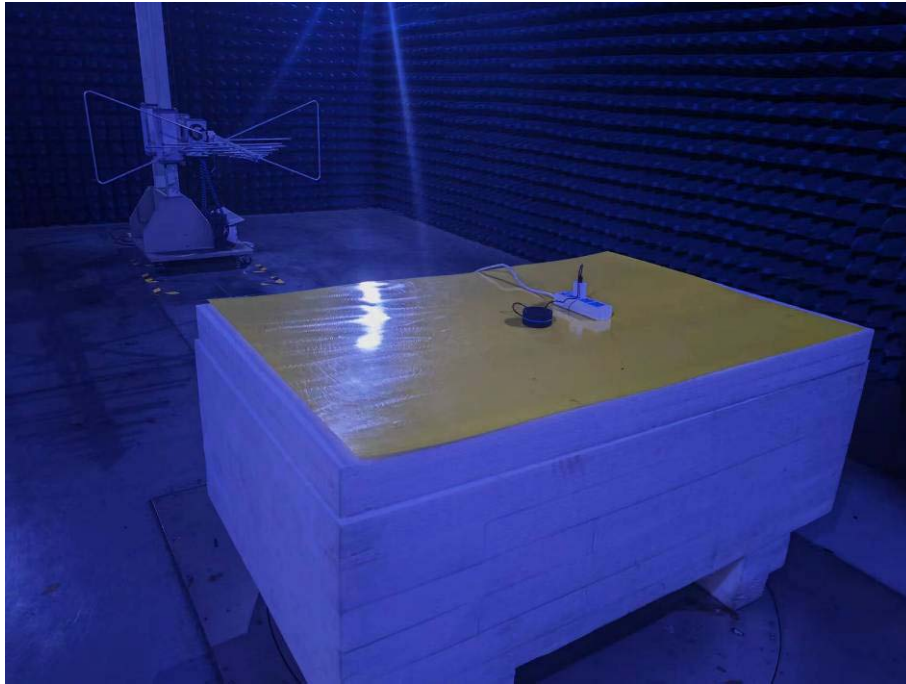
Photo of Radiated Emission Measurement Below 1GHz
