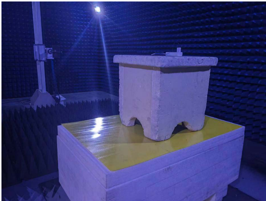
Photo of Radiated Emission Measurement Above 1GHz
