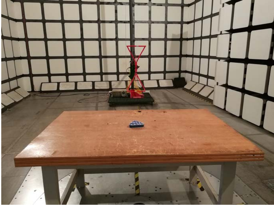
Radiated Emissions View (Below 1 GHz)
