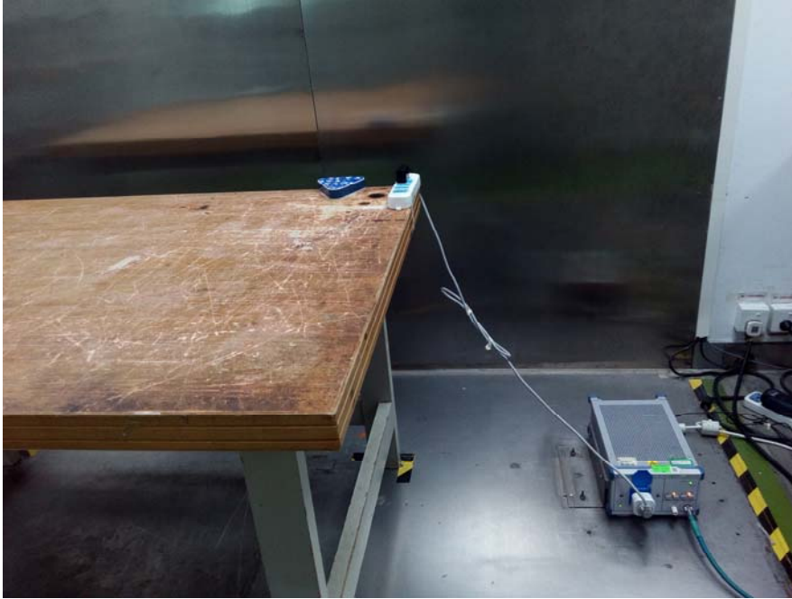
Conducted Emissions - Front View
