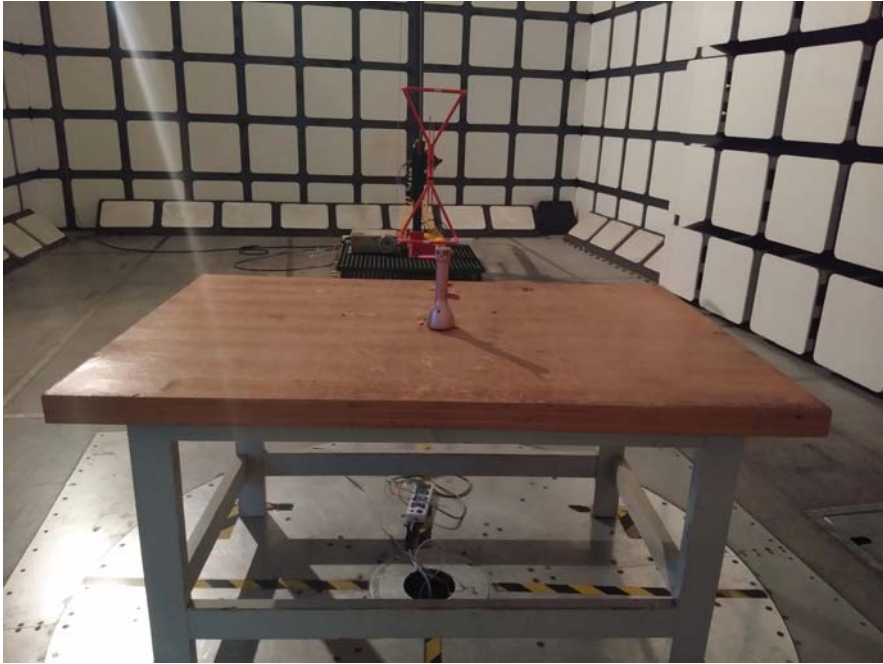
Radiated Emissions View (Below 1 GHz)
