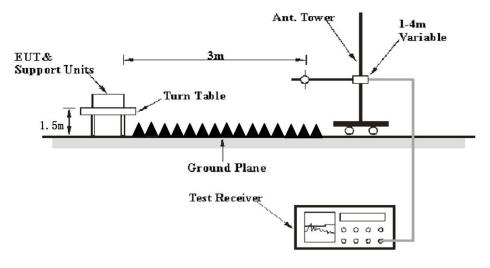
The radiated emission tests were performed in the 3 meters, using the setup accordance with the ANSI C63.10-2013. The specification used was the FCC 15.209 and FCC 15.247 limits.
