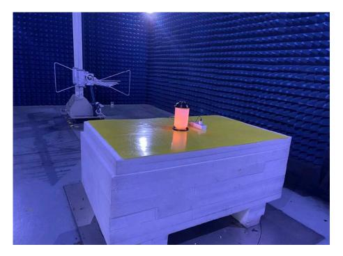
**Radiated Spurious Emissions Test View (Below 1GHz)**
