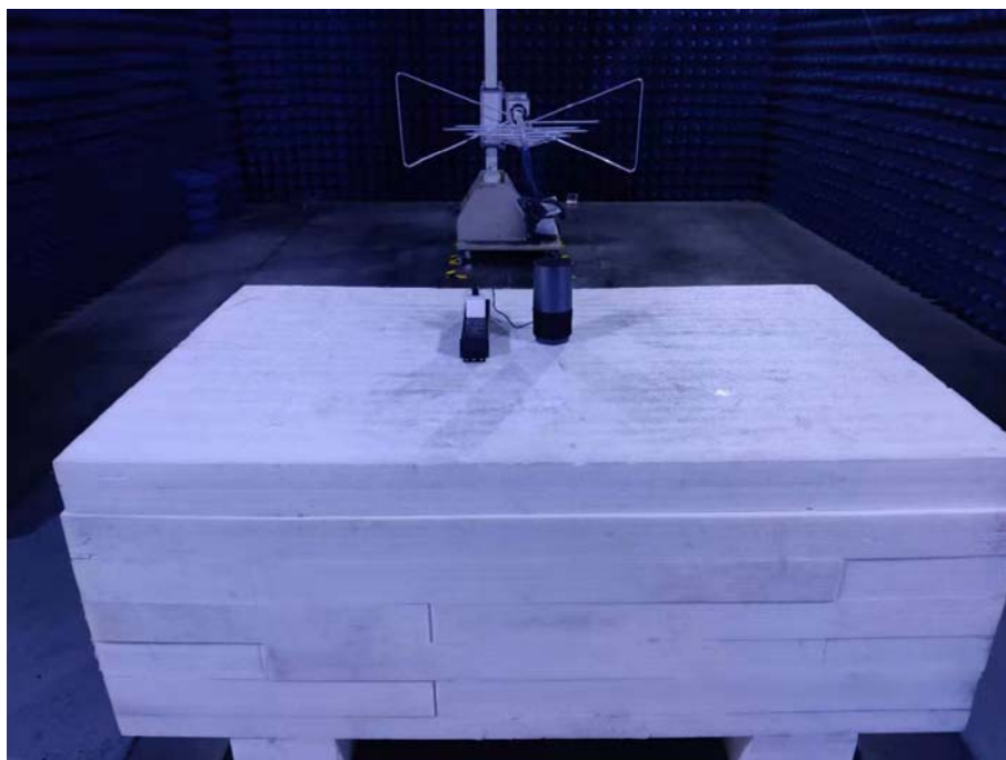
Photo of Radiated Emission Measurement Above 1GHz
