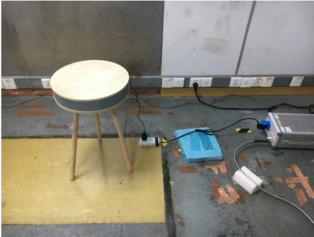
Photo of Conducted Emission Measurement
