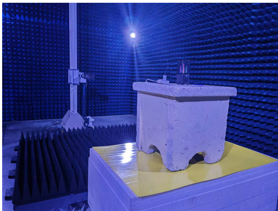
Photo of Radiated Emission Measurement (Above 1G)
