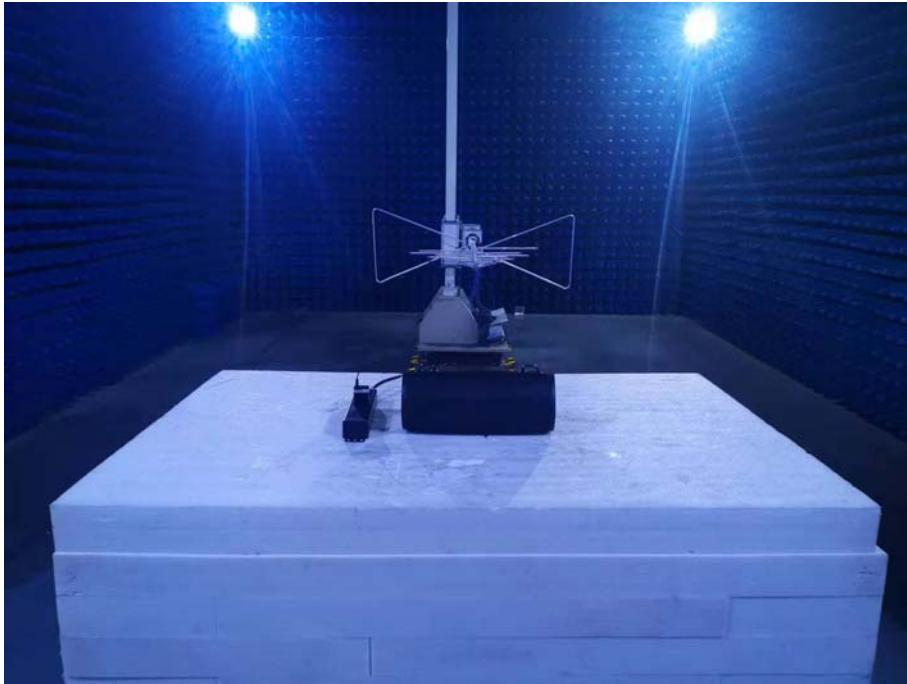
Photo of Radiated Emission Measurement Below 1GHz
