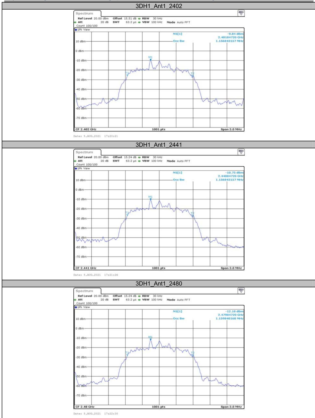
**Appendix C: Maximum conducted Peak output power****Test Result**
