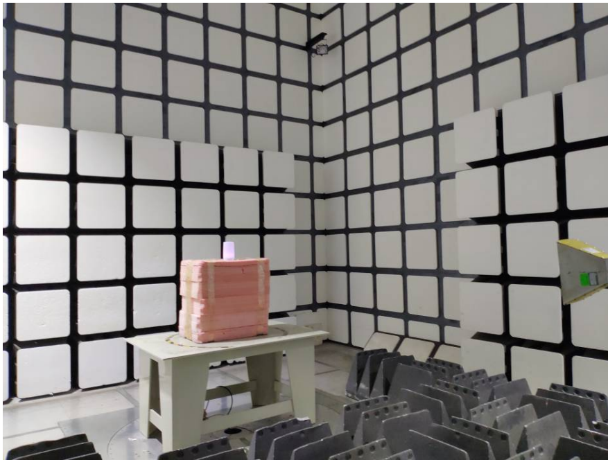
Radiated Emissions View (Above 1 GHz)
