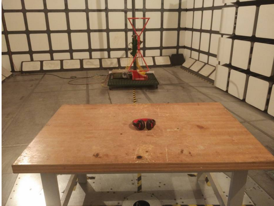
Radiated Emissions View (Below 1 GHz)
