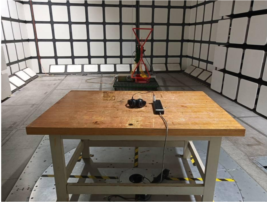
Radiated Emissions View (Below 1 GHz)
