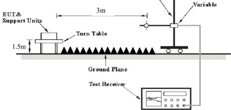
The radiated emission performed in the 3 meters, using the setup accordance with the ANSI C63.10-2013. The specification used was the FCC 15.209, FCC 15.247 limits.
