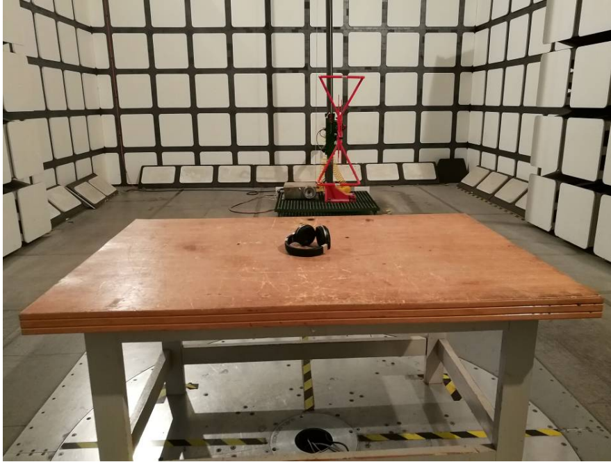
Radiated Emissions View (Below 1 GHz)
