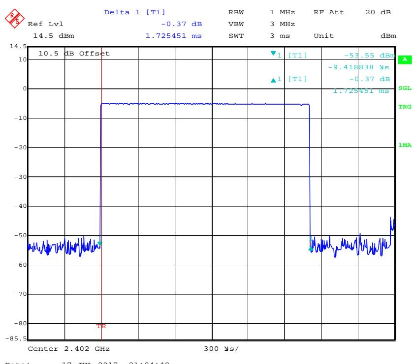
**Pulse time, Middle Channel, DH3**
