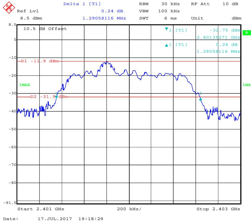
**EDR (8DPSK): Middle Channel**
