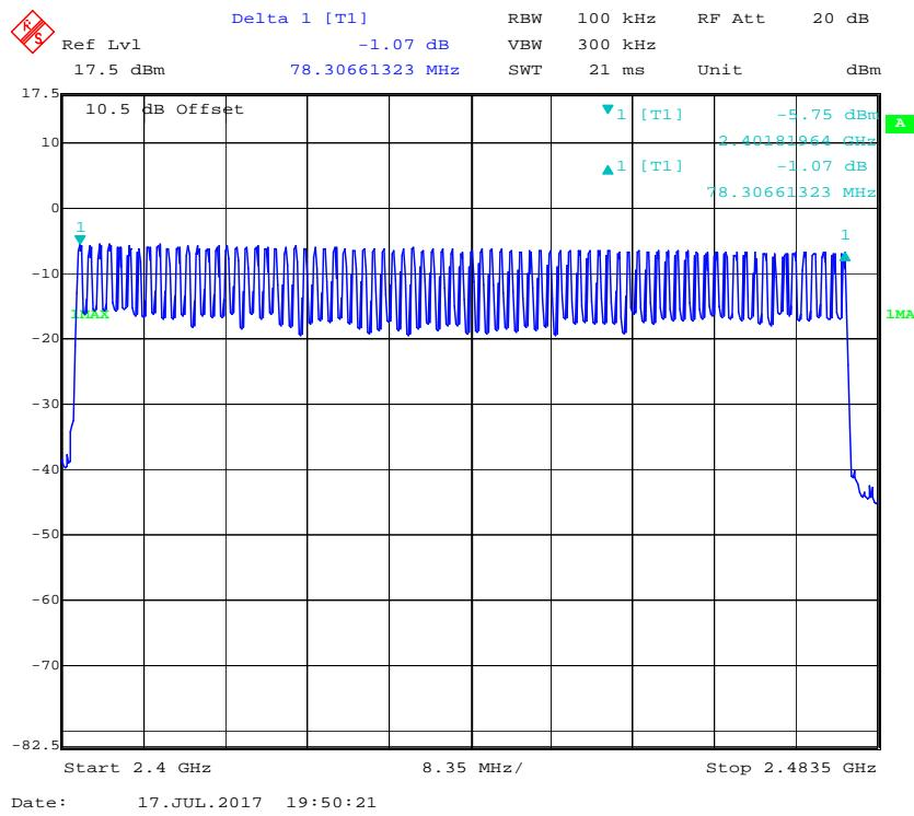
**EDR ( $\pi/4$ -DQPSK): Number of Hopping Channels**
