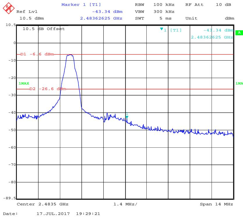
**EDR ( $\pi/4$ -DQPSK): Band Edge-Left Side**
