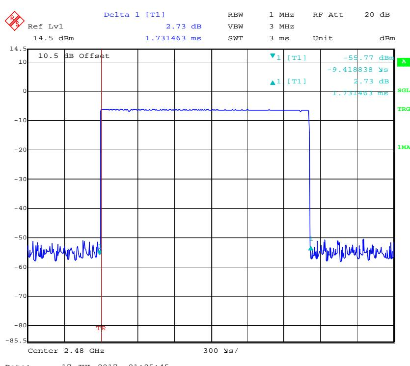
**Pulse time, Low Channel, DH5**
