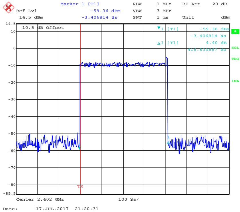
**Pulse time, Middle Channel, 2DH1**
