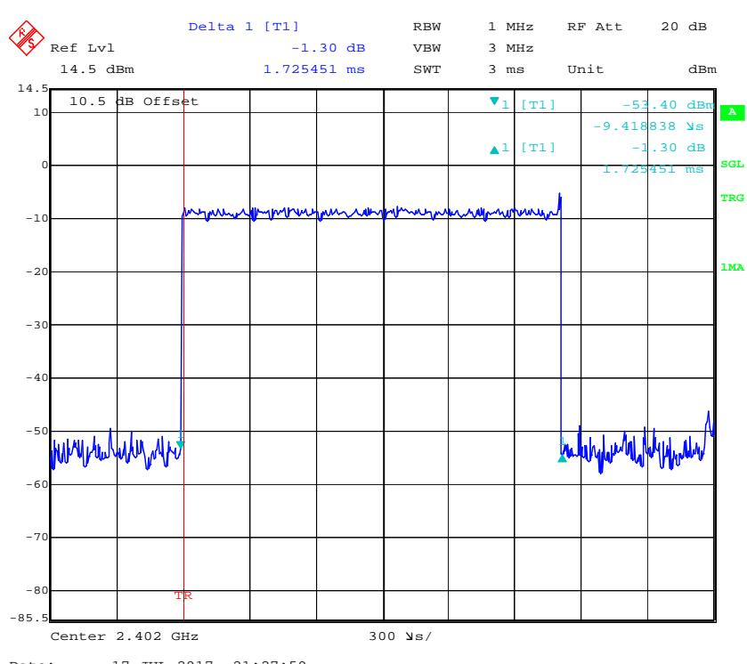
**Pulse time, Middle Channel, 3DH3**
