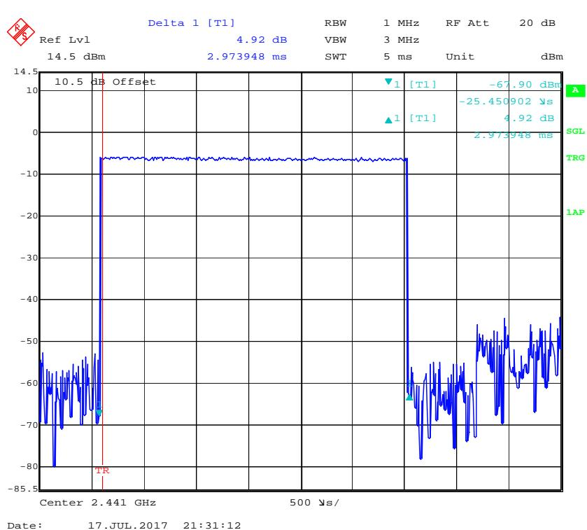
**Pulse time, High Channel, DH5**
