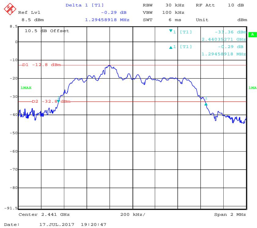
**EDR ( $\pi/4$ -DQPSK): High Channel**
