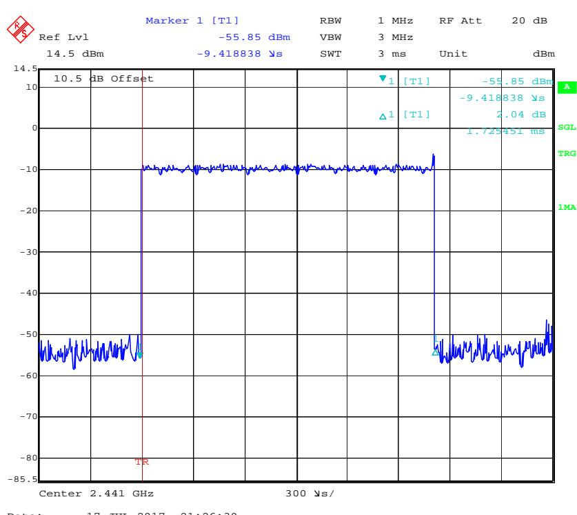
**Pulse time, High Channel, 2DH3**
