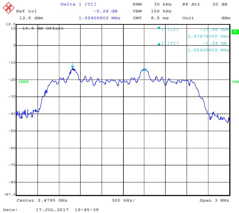
**EDR (8DPSK): Low Channel**
