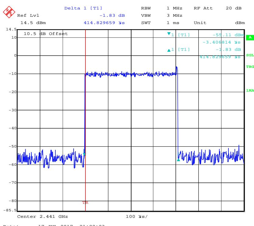
**Pulse time, High Channel, 3DH1**
