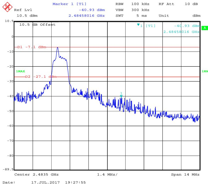
**EDR (8DPSK): Band Edge-Left Side**
