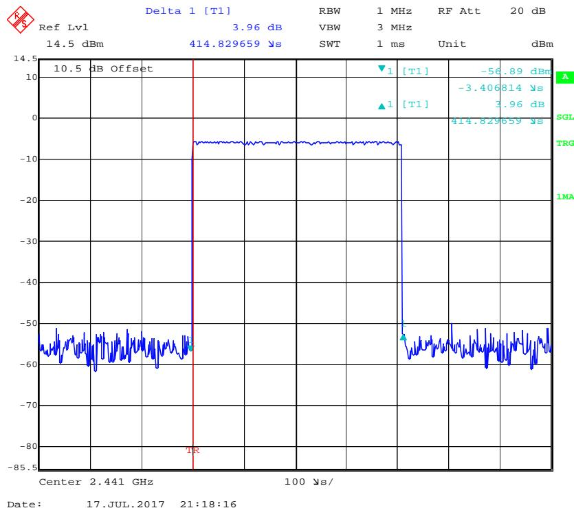
**Pulse time, High Channel, DH1**
