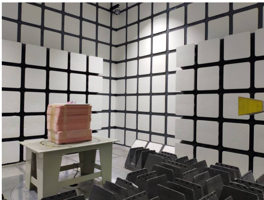
Radiated Emissions View (Above 1 GHz)
