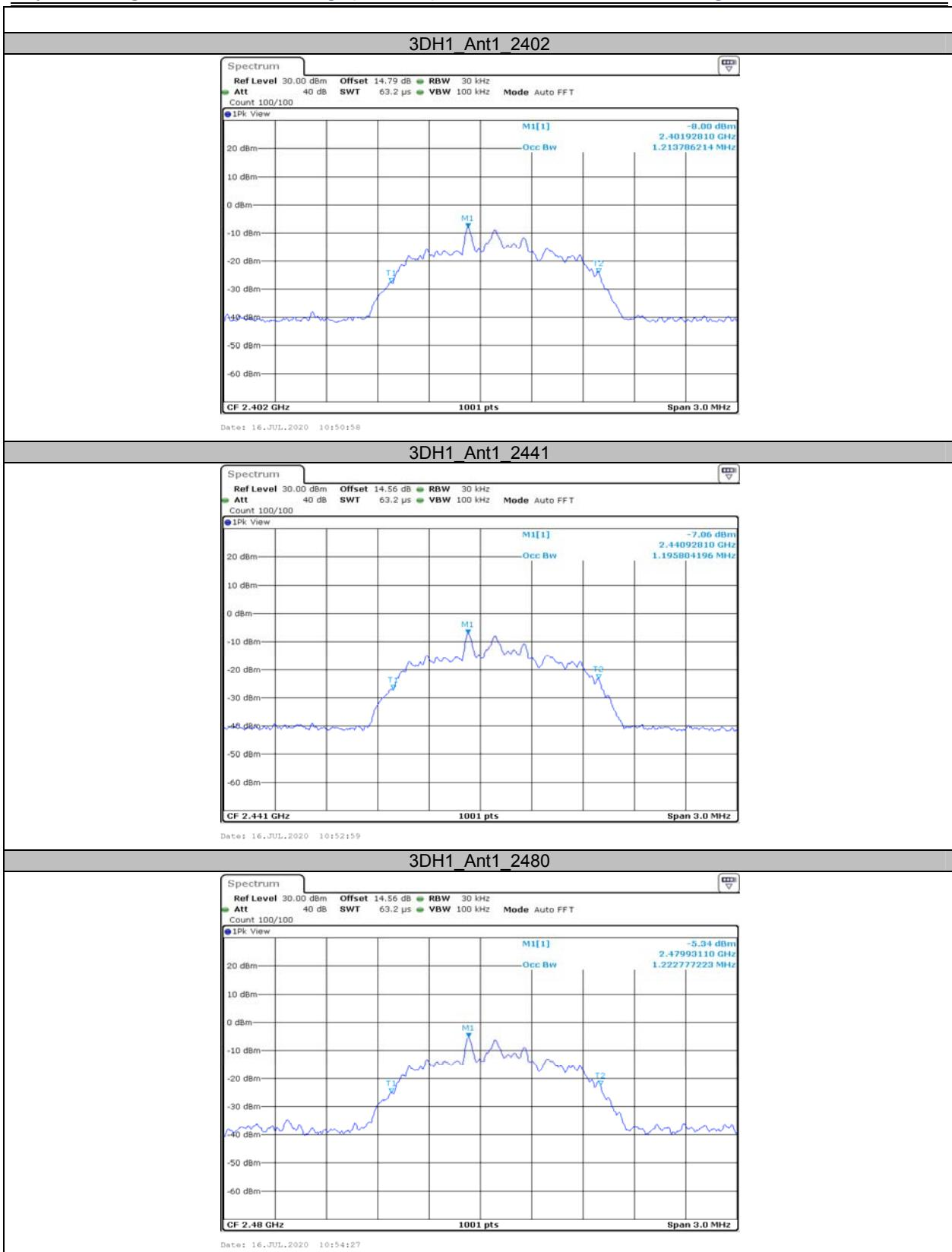
**Appendix C: Maximum conducted Peak output power****Test Result**
