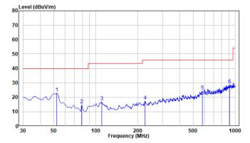
Site : chamber Condition: 3m VERTICAL Job NO. : SZNS211103-56531-RF Mode : TX
