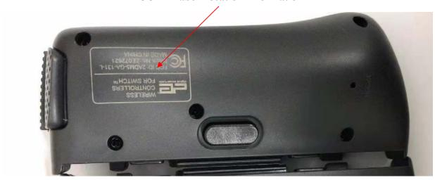
The label shown shall be permanently affixed at a conspicuous location on the device and be readily visible to the user at the time purchase (Labeling requirements per 2.925)
