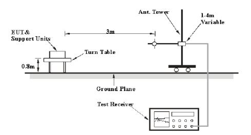
The radiated emission tests were performed in the 3 meters, using the setup accordance with the ANSI C63.10-2013. The specification used was the FCC Part 15.205 and 15.209 and 15.229 limits.
