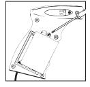
To install batteries into the Gesture Remote Control, unscrew the screw on the battery box cover to open the battery compartment. Insert 3 x "AAA" 1.5V batteries (Not Included) into the battery box. Batteries should be placed as shown on the diagram.
