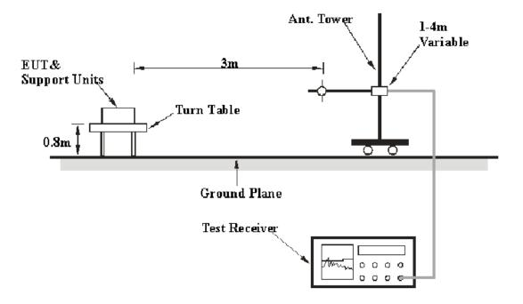
The radiated emission tests were performed in the 3 meters, using the setup accordance with the ANSI C63.10-2013. The specification used was the FCC Part 15.205 and 15.209 and 15.227 limits.
