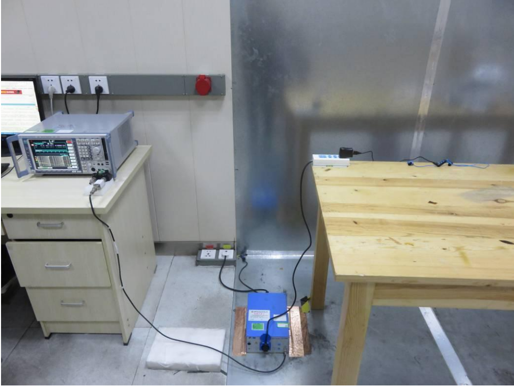
FCC RADIATED EMISSION TEST SETUP
