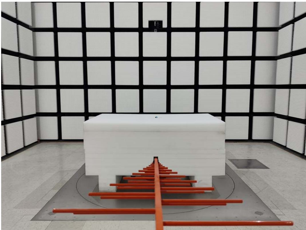
Radiated Emission Below 1GHz View Right
