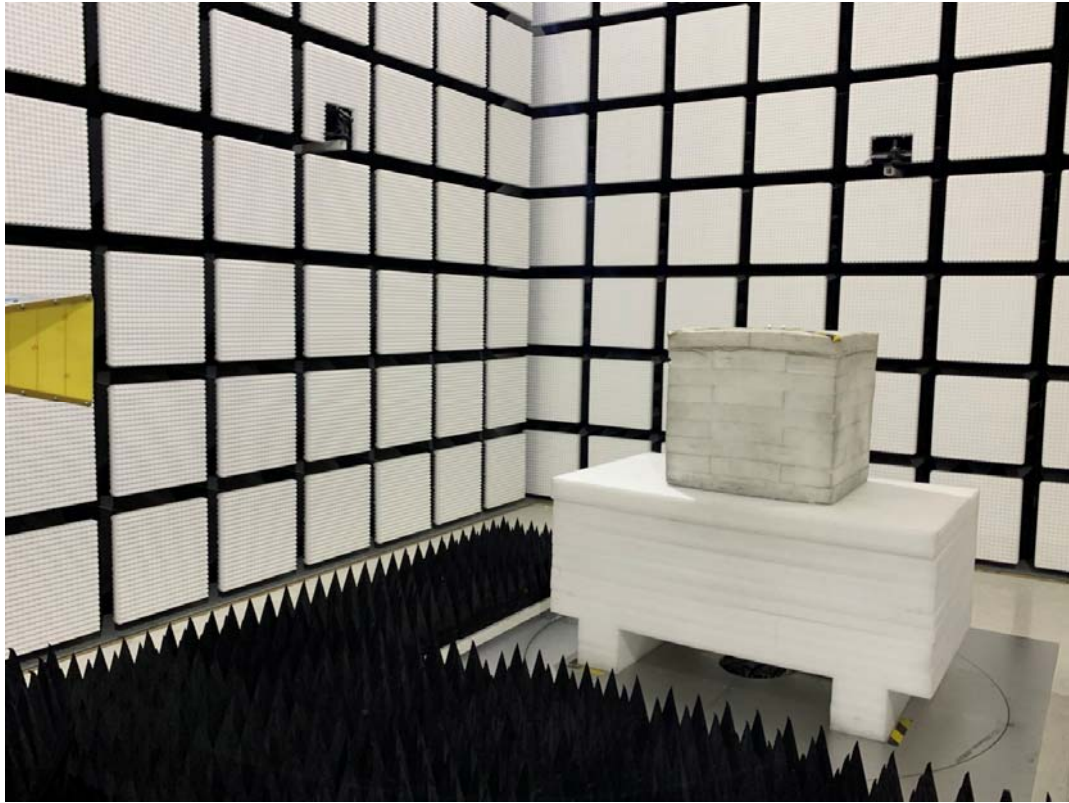
Radiated Emission Above 1GHz View Left
