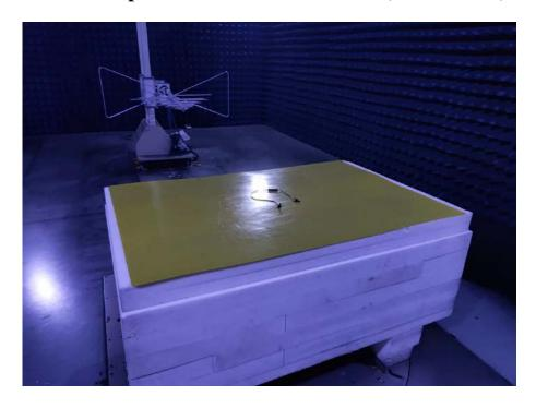
**Radiated Spurious Emissions Test View (Above 1GHz)**
