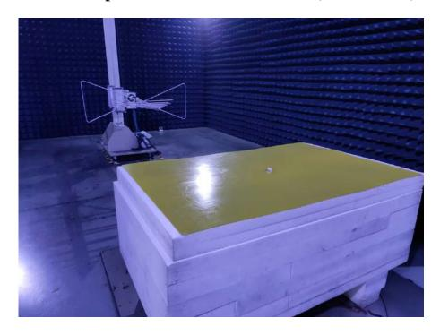
**Radiated Spurious Emissions Test View (Above 1GHz)**
